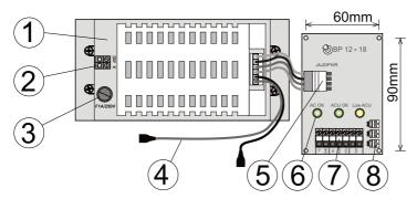
Figure: 1 - JA-83PWR transformer, 2- input voltage terminals 230 V, 3 - fuse for AC circuit (1.6 A), 4 - backup battery connector, 5 - link of JA-83PWR to the BP12-18, 6 - indication LEDs, 7 - output voltage terminals, 8 - tamper input connectors (3x)
